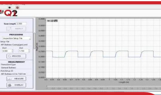
THREAD PROFILE GEOMETRY: DISPLAYS ALL THREADS THAT WERE SCANNED
