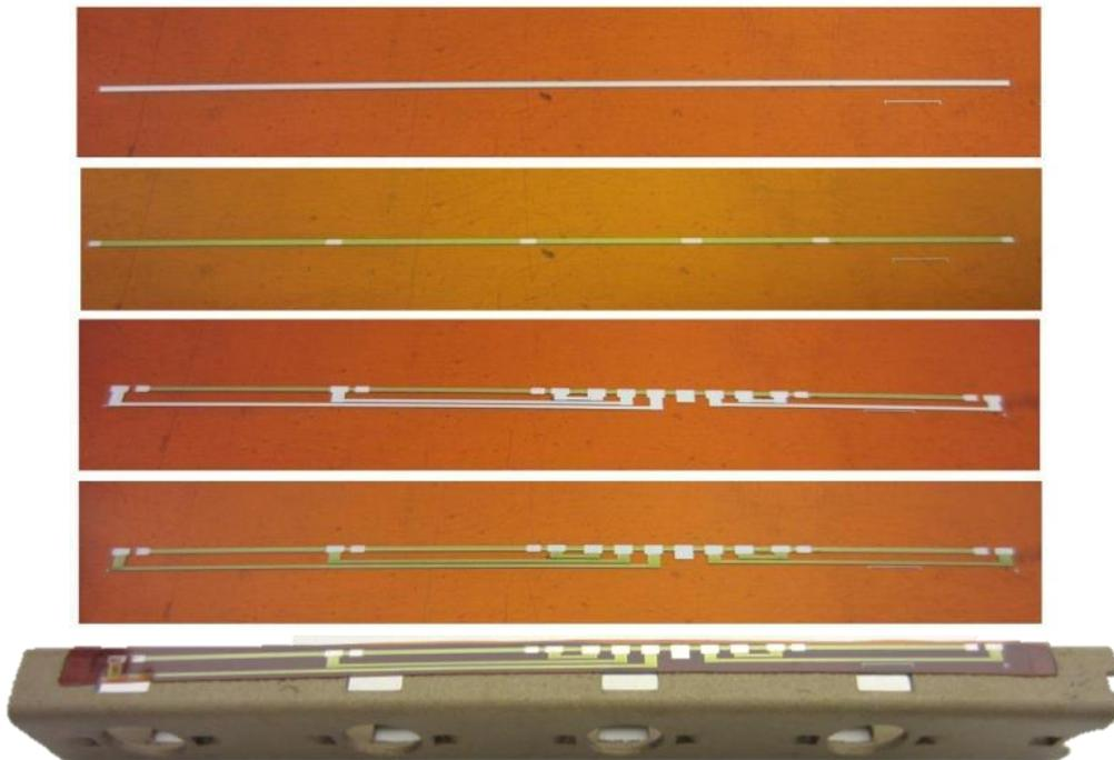
**Figure 6.** Serial images of AJ printed multi-layer flex circuit and final mounting to part
