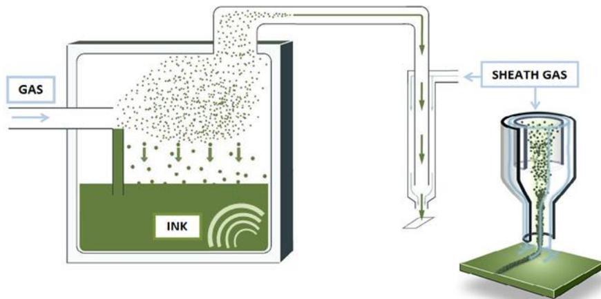
**Figure 1.** Detailed schematic of Aerosol Jet technology in which aerosolized ink is focused over a 5 mm standoff. (Figure courtesy of Optomec, Inc.)
