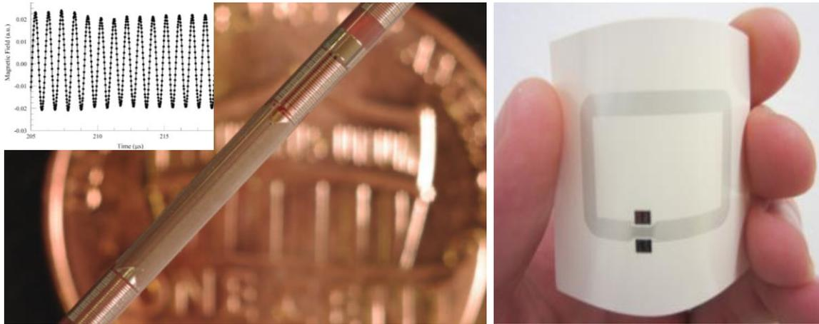
**Figure 10.** (L) Three-channel, three-axis conformal probe on 1.4 mm diameter tube<sup>6</sup> over a penny, (R) RFID coil on paper
