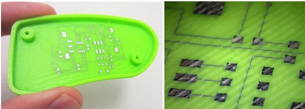
**Figure 5.** (L) Printed circuit on ABS printed case, (R) enhance view of printed ABS surface
