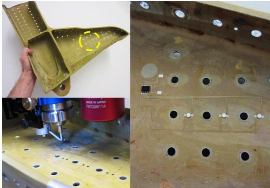
**Figure 2.** (Top left) F-15 component, (Bottom left) deposition of monitoring circuit, (R) final product. Concept developed by Qi2.
