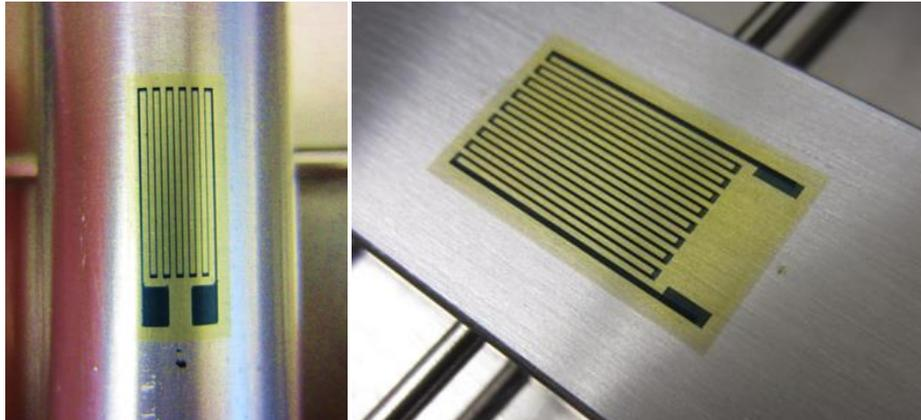
**Figure 4.** (L) Strain gauge on stainless steel pipe, (R) SG on aluminum bar
