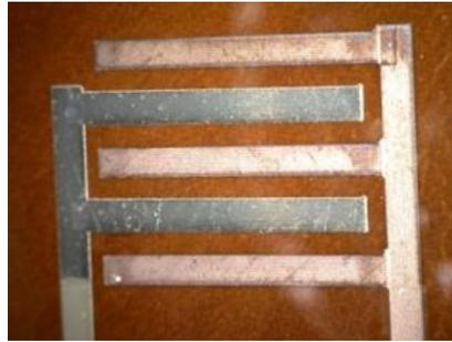
**Figure 8.** Interdigitated water sensor consisting of Ag-Cu electrodes (Ag – left, Cu – right).
