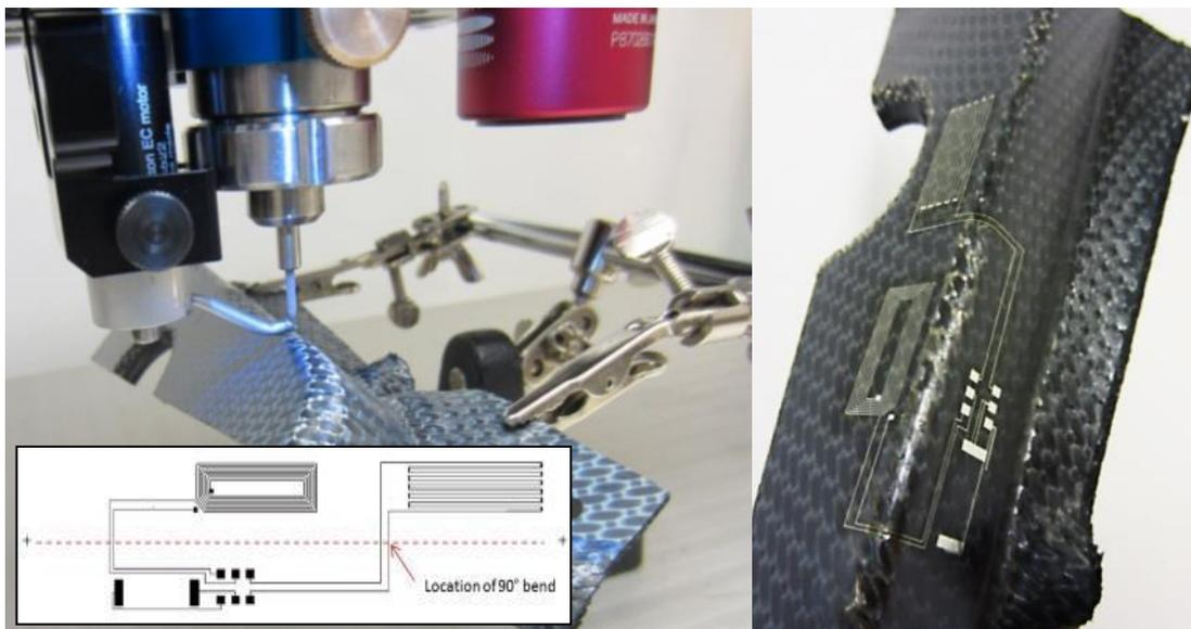
**Figure 3.** (L) Composite oriented in a clamp fixture with the associated CAD layout (inset), (R) printed circuitry and strain gauge. Concept developed by Qi2.
