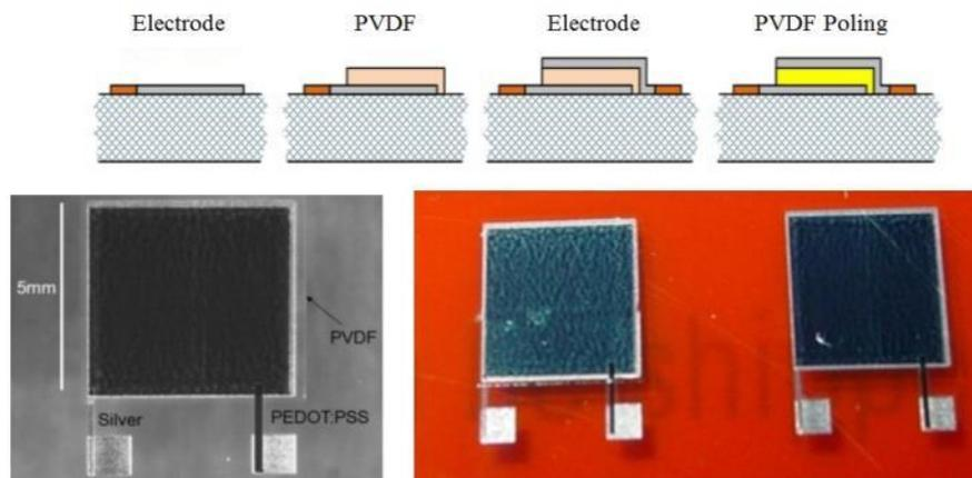
**Figure 7.** (Top) Sketch of fabrication process for direct-write pressure transducer, (Bottom left) Illustrated transducer on glass, (Bottom right) PVDF transducer printed on Kapton foil.
