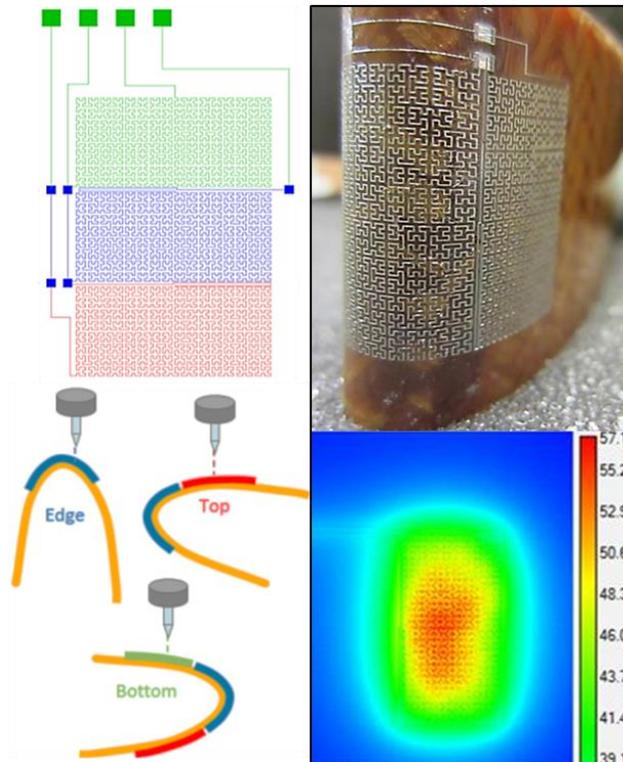
**Figure 9.** (L) Heater pattern in color to illustrate serial printed segments, (Top right) Printed top side and leading edge, (Bottom right) Thermal IR image of printed heater.
